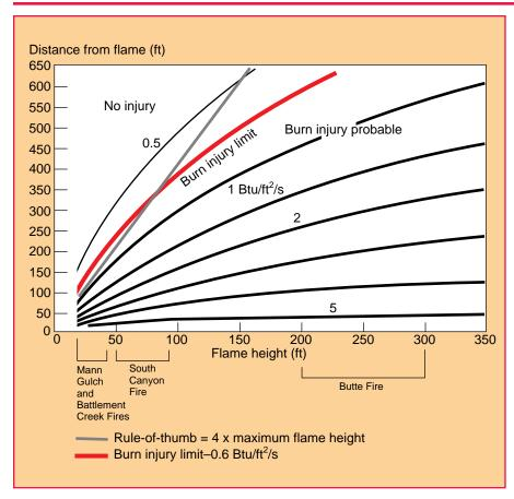
**Figure 1**—Lines represent predicted radiant energy arriving at the firefighter as a function of flame height and distance from the flame. It is assumed that the firefighter is wearing fire-retardant clothing and protective head and neck equipment. The heavy shaded line represents the burn injury threshold of 0.6 Btu/ft²/s (7 kW/m²). The heavy solid black line indicates the rule of thumb for the size of the safety zone.
