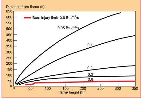
**Figure 2**—Predicted radiant energy on a fire shelter as a function of distance between the fire shelter and flames, and flame height. The heavy shaded line represents the burn injury threshold for a firefighter inside a deployed fire shelter.
